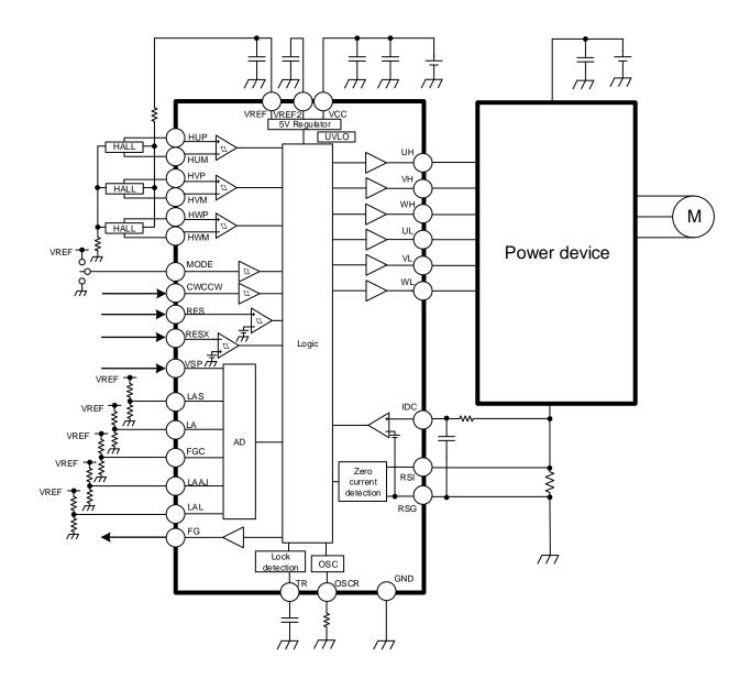
Note: The RESX pin and VREF pin are only in TC78B042FTG.
