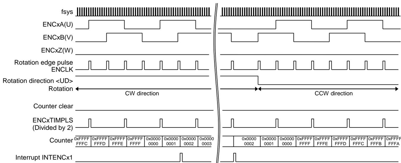
**Figure 3.4 2-phase decode ( $[ENxTNCR] \langle P3EN \rangle = 0$ )**
