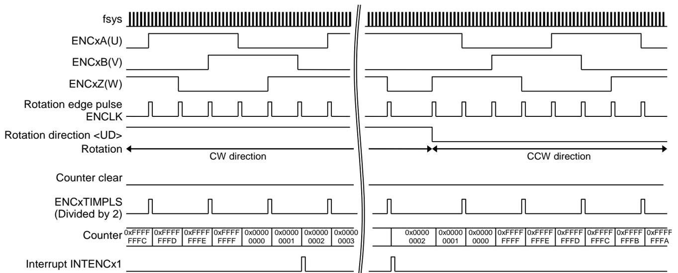
Figure 3.3 3-phase decode ( $[ENxTNCR] \langle P3EN \rangle = 1$ )
