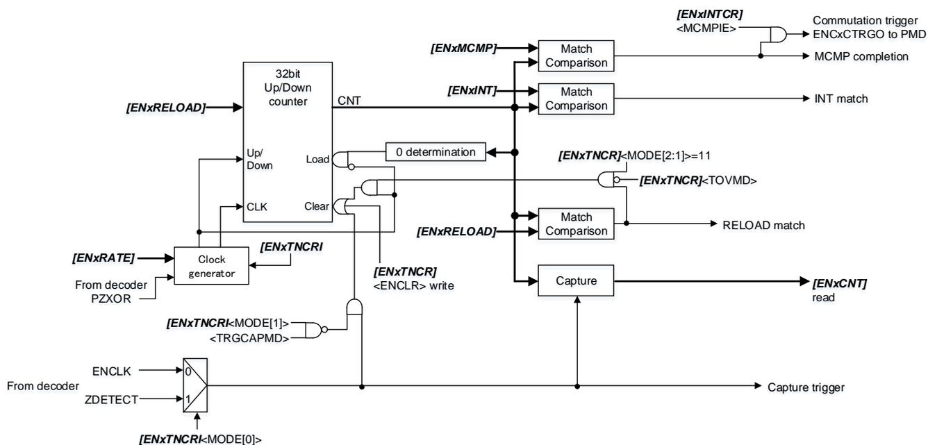
**Figure 3.24 Counter configuration (Sensor mode (Phase count) and Phase counter mode)**
