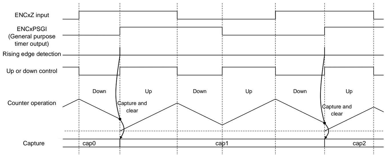
**Figure 3.13 Operation of Phase counter mode (Phase difference)**
