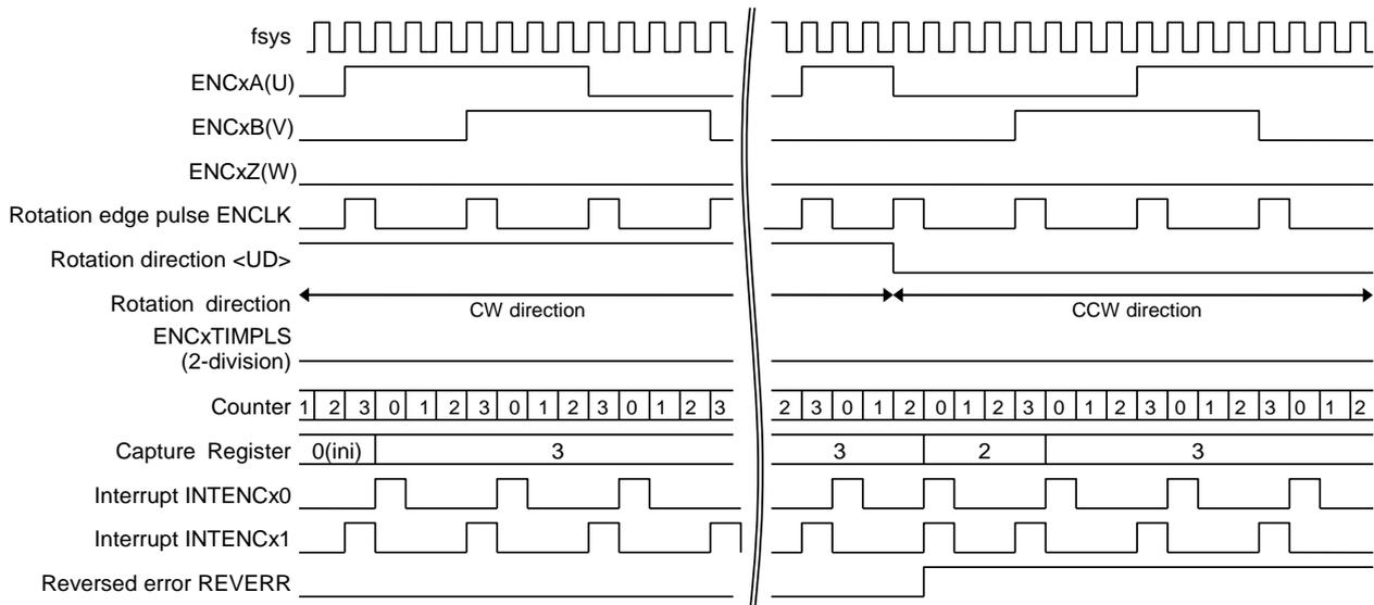
Figure 3.6 2-phase decode ( $[ENxTNCR]<P3EN> = 0$ )
