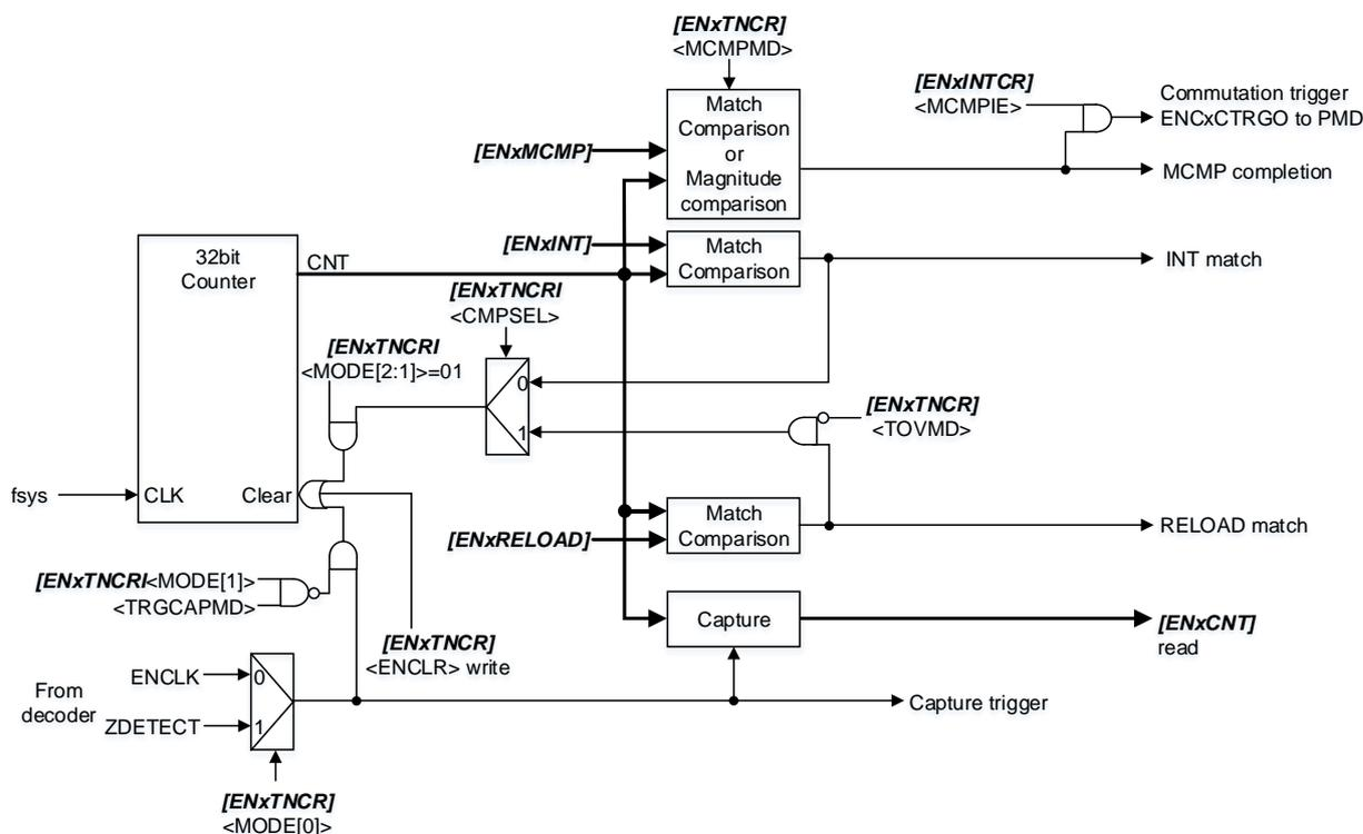
**Figure 3.23 Counter configuration (Sensor mode (Timer count) and Timer mode)**
