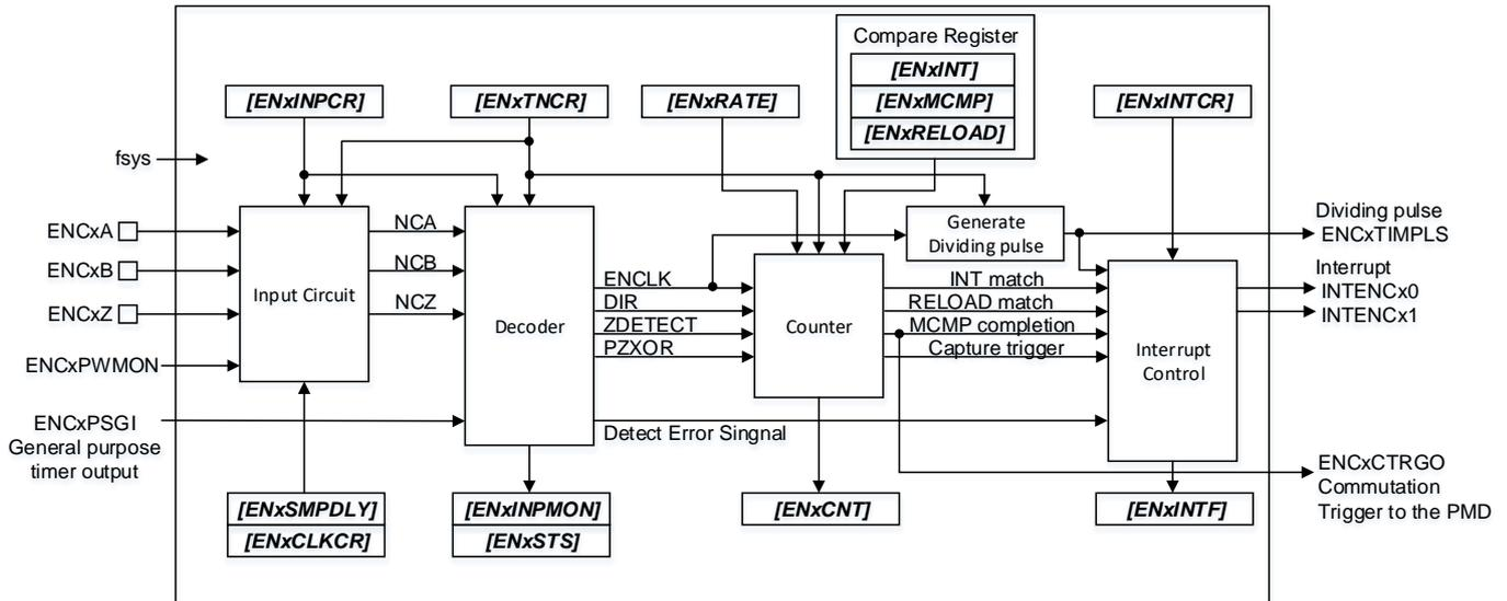
Figure 2.1 Block diagram of A-ENC32-A
