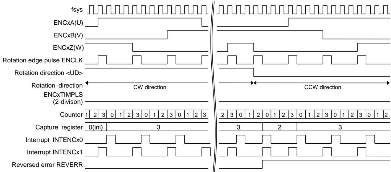
Figure 3.5 3-phase decode ( $[ENxTNCR]<P3EN> = 1$ )
