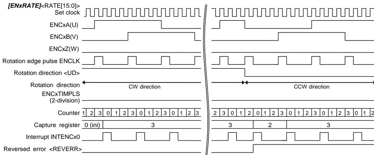
Figure 3.8 2-phase decode ( $[ENxTNCR]<P3EN> = 0$ )
