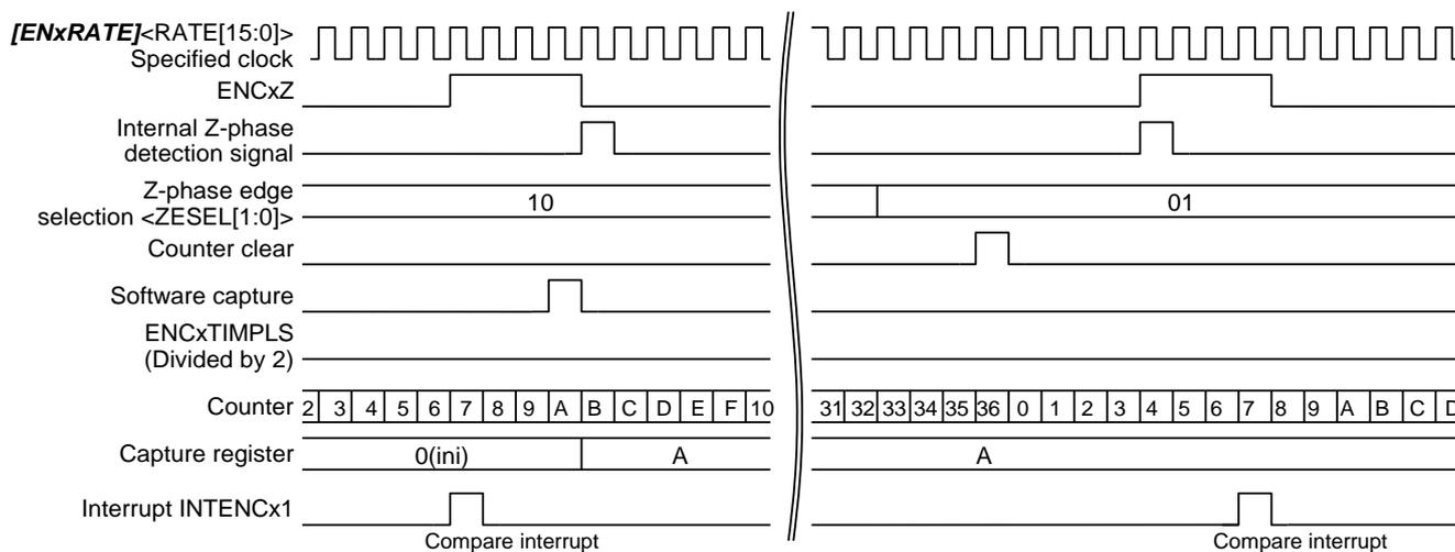
**Figure 3.12 ENCxZ input is invalid ( $[ENxTNCR]\langle ZEN \rangle = 0$ )**
