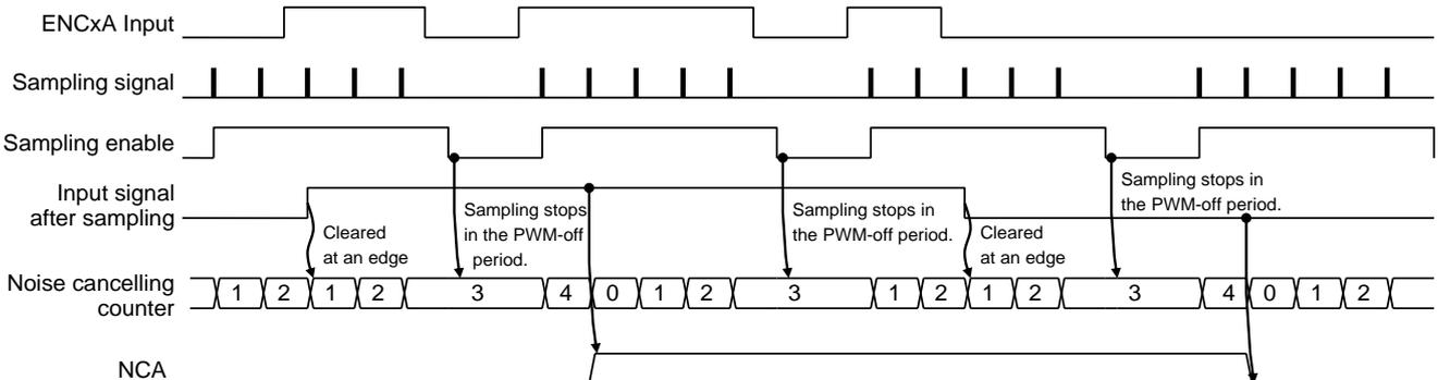
**Figure 3.17 Noise cancelling (PWM-On period sampling and PWM-Off period stop:
