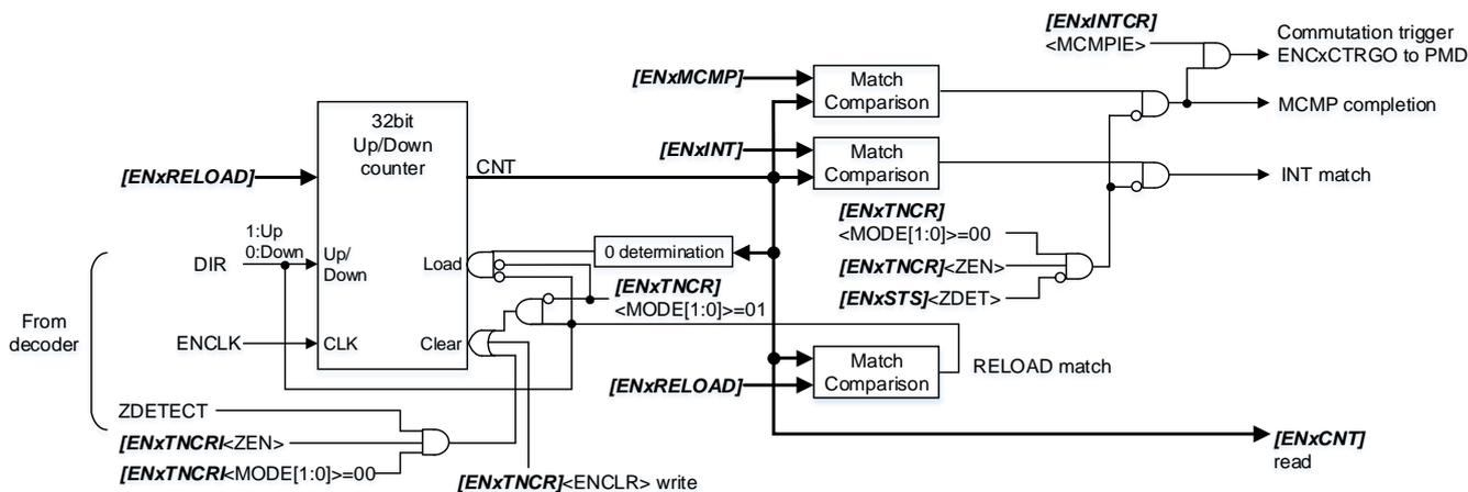
Figure 3.22 Counter circuit (Encoder mode and Sensor mode (Event count))
