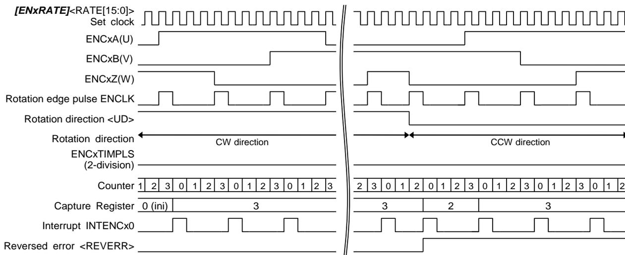
Figure 3.7 3-phase decode ( $[ENxTNCR]<P3EN> = 1$ )
