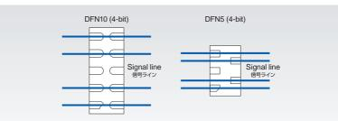
Multibit TVS diode arrays are suitable for use in USB and other buses consisting of multiple signal lines. The flow-through pinout simplifies board layout.
