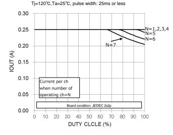
IOUT-DUTY CYCLE Mounted on the board of TBD62502AFNG/TBD62503AFNG Tj=120°C,Ta=25°C, pulse width: 25ms or less 0.30 N=1,2 0.25 N=3 N=40.20 N=5 IOUT (A) N=6 N=7 0.15 0.10 Current per ch when number of operating ch=N 0.05 rd condition:  $50 \times 50 \times 1.6$  mm Cu 40% , single-side glass epoxy 0.00 10 20 30 40 50 60 70 80 90 100 DUTY CYCLE (%)
