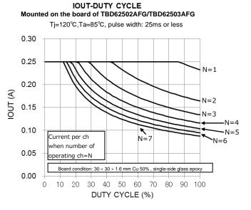
IOUT-DUTY CYCLE Mounted on the board of TBD62502AFWG/TBD62503AFWG
