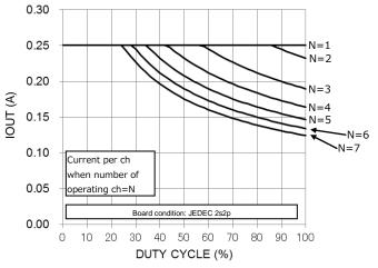
IOUT-DUTY CYCLE Mounted on the board of TBD62502AFNG/TBD62503AFNG
