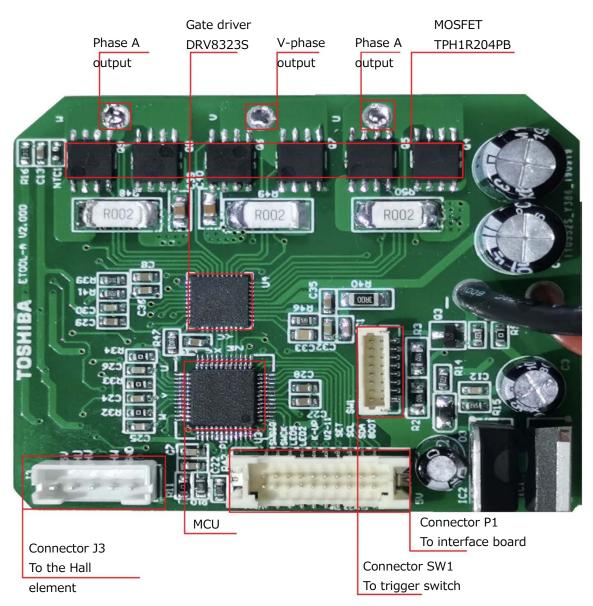
Fig.5.1 Layout of the Main Board
