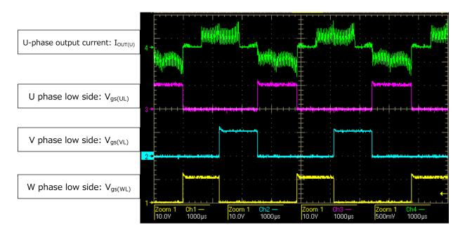
Fig.6.3 Square Wave Drive Mode Operation Waveforms (2)
