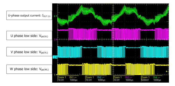
Fig.6.5 Sine Wave Drive Mode Operation Waveforms (2)
