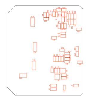
Fig.4.4 Main Board Substrate Silk (Bottom side)
