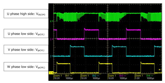
Fig.6.2 Square Wave Drive Mode Operation Waveforms (1)
