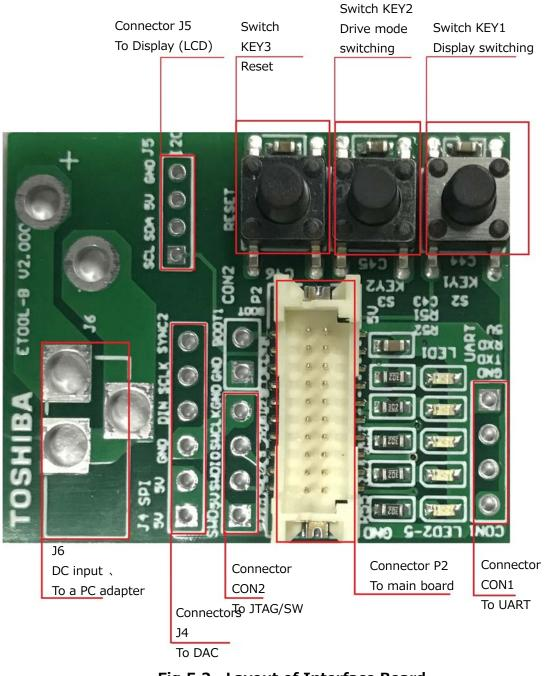
Fig.5.2 Layout of Interface Board
