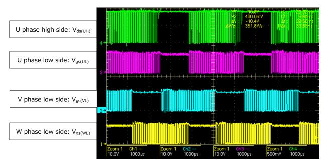
Fig.6.4 Sine Wave Drive Mode Operation Waveforms (1)
