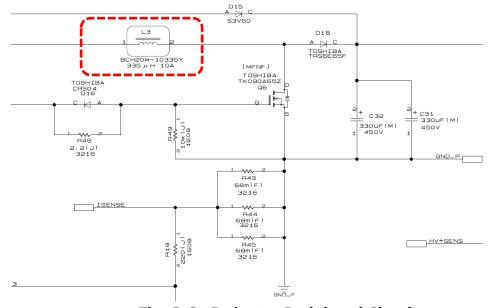
Fig. 2.6 Inductor Peripheral Circuit
