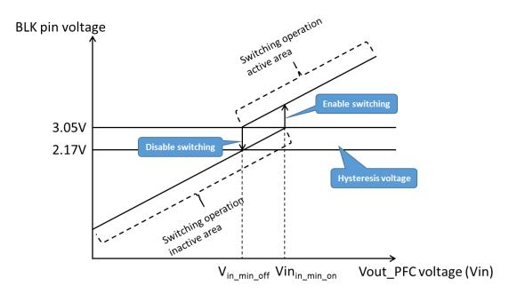
Fig. 2.11 Input Voltage vs BLK Pin Voltage, Switching Operation Status
