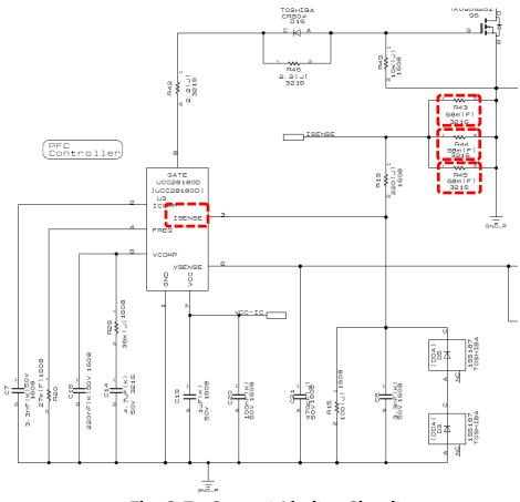
Fig. 2.7 Current Limiter Circuit
