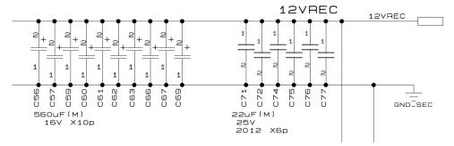
Fig. 2.20 Output Capacitor Circuit
