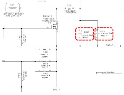
Fig. 2.8 Output Capacitor Peripheral Circuit
