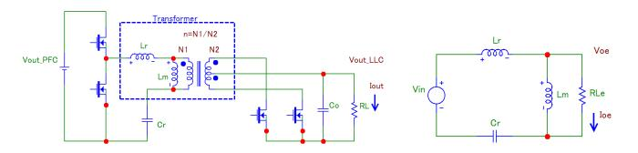
Fig. 2.13 LLC Resonant Basic Circuit
