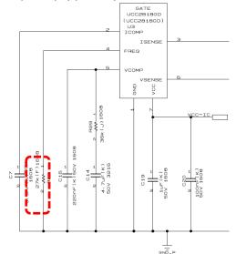
Fig. 2.5 Switching Frequency Adjustment Circuit
