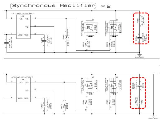
Fig. 2.21 Snubber Circuit
