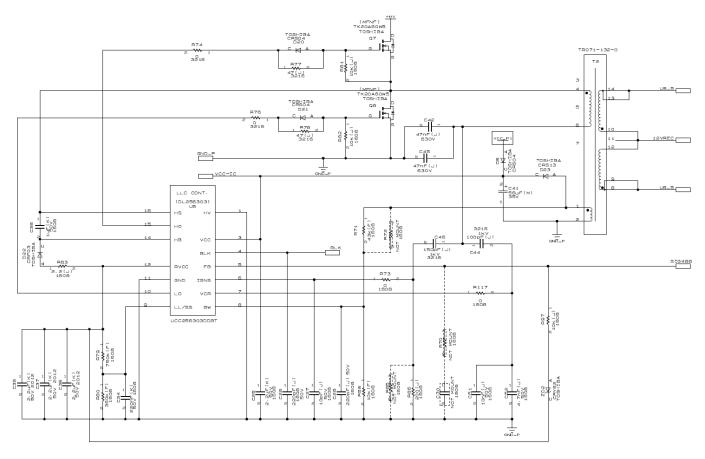
Fig. 2.9 LLC Circuit (Around the LLC Controller)
