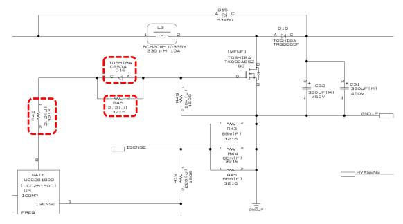
Fig. 2.4 Gate Drive Circuit
