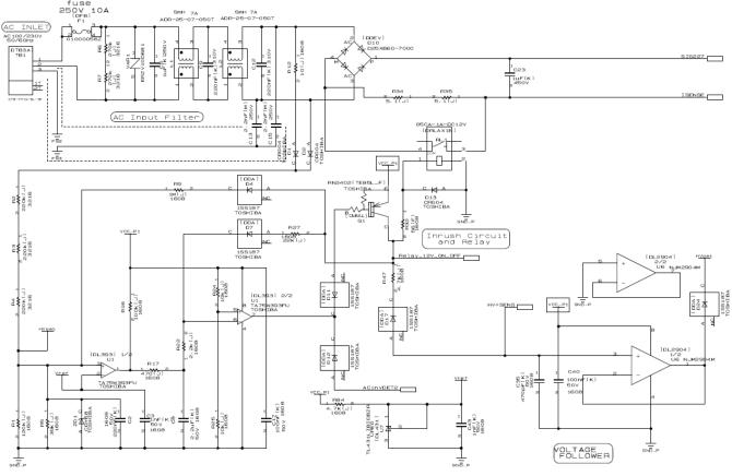
Fig. 2.1 AC Line Circuit
